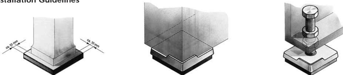
In order to obtain optimal stabilisation of the machine, it is recommended to allow the ISOCOL plates to protrude approx. 10 mm from the machine base. The single plates must be mounted such that the load is evenly distributed.
