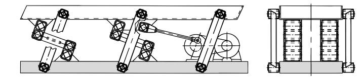
The oscillating conveyor systems are built such that they run very close to the resonance frequency in order to keep the energy consumption down and to improve the fatigue resistance of the structure (trough and frame). The total spring value  $c_t$  of the trough should be approximately equal to
