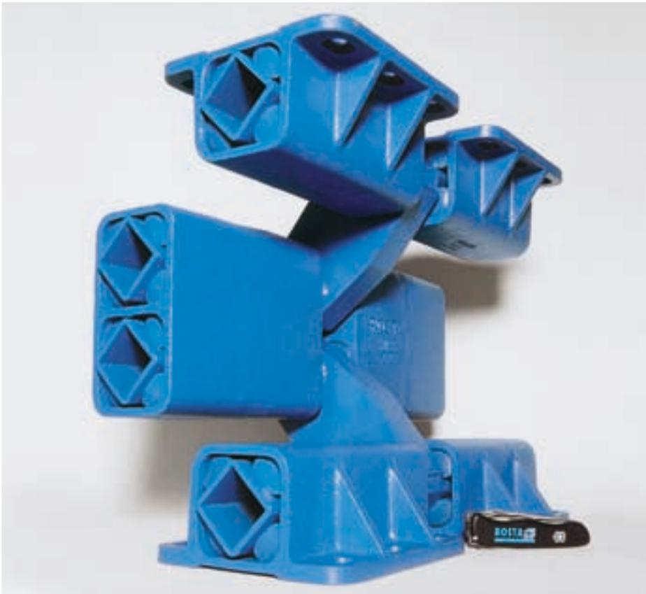
ROSTA Oscillating Mountings Type AB 50 «TWIN» were developed for the suspension of large-scale screens. Types «TWIN» 50 and 50-2 possess the same impressive characteristics as the smaller sizes of the ROSTA screen suspension series AB, but have a significantly higher loading capacity: Type AB 50 «TWIN» = 12 000 N and the version AB 50-2 «TWIN» = 20 000 N.
