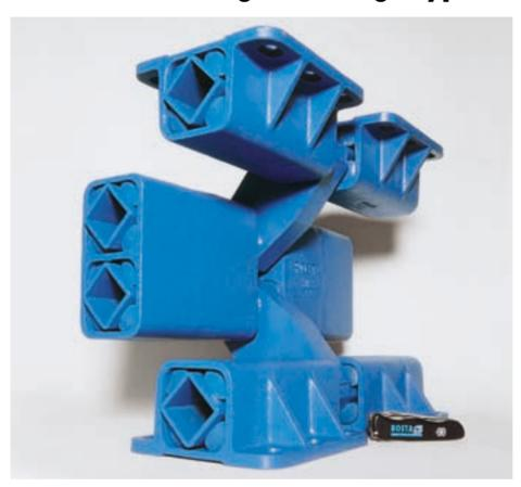
ROSTA Oscillating Mountings Type AB 50 «TWIN» were developed for the suspension of large-scale screens. Types «TWIN» 50 and 50-2 possess the same impressive characteristics as the smaller sizes of the ROSTA screen suspension series AB, but have a significantly higher loading capacity: Type AB 50 «TWIN» = 12 000 N and the version AB 50-2 «TWIN» = 20 000 N.
