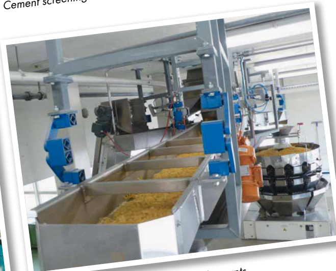
Pasta-feeding-channel hanging on HS-mounts
