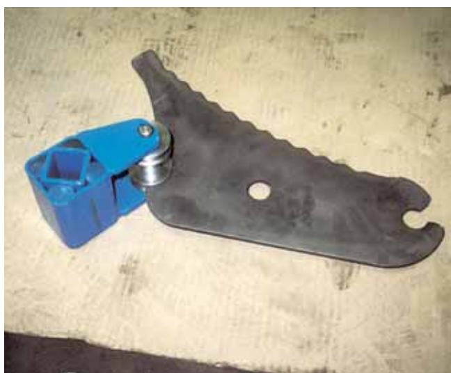
Elastic suspension of shaping knife in baler
