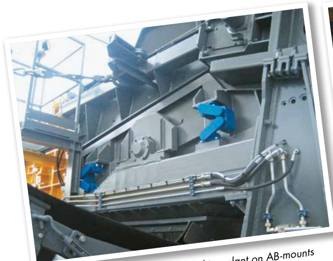
Fluid-bed-cooler on AB-D-mounts
