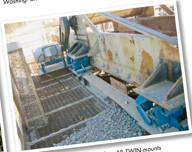
Washing- and dewatering-screen for vegetables on AB-mounts
