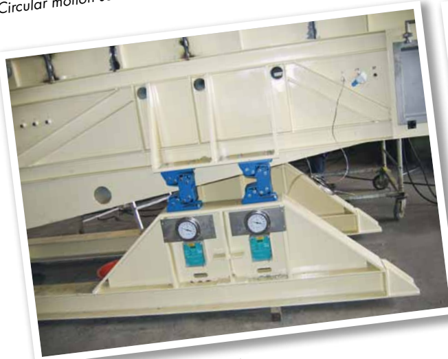
Fluid-bed-cooler on AB-D-mounts
