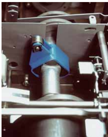
Elastic stop to absorb high impacts
