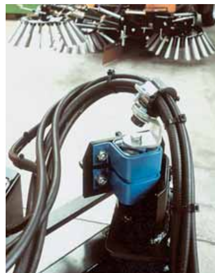
Suspension of a brush in road sweeper
