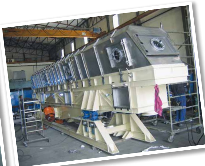
Fluid-bed-cooler on AB-D-mounts
