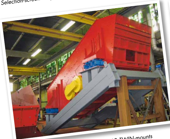
Selection-screen for potato chips on stainless steel AB-mounts
