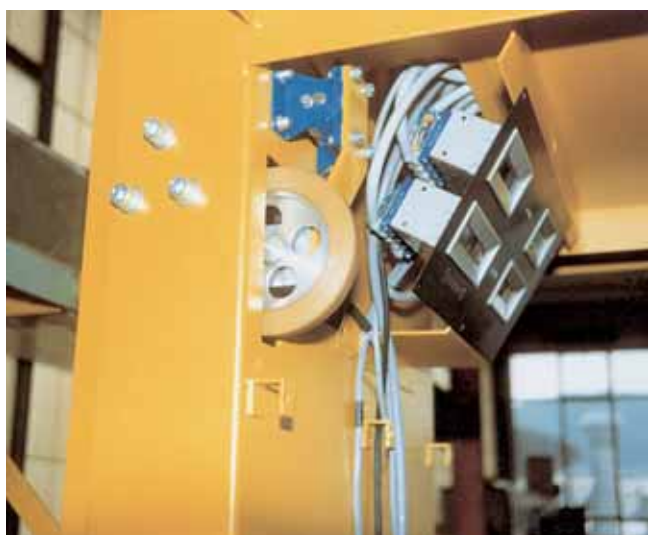
Elastic suspension of caliper roll in elevator
