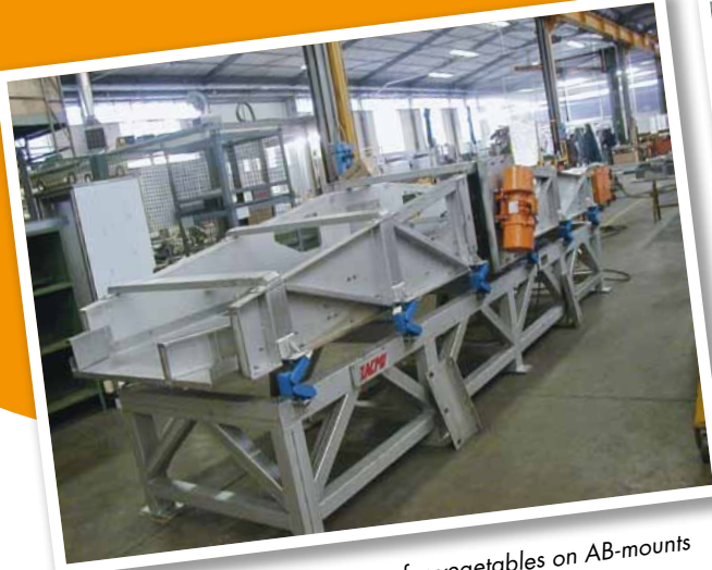
Vegetable-feeder on stainless steel AB-mounts
