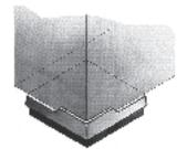
In case there is no levelling necessary it is possible to push the ISOCOL U elements directly under the machine base, up to the retaining edge. Additional fixation is not necessary.
