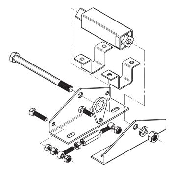
The drawing on the left shows the construction of the ROSTA Motorbase MB 27. Contrary to the large type MB 50 and MB 70, the MB 27 Motorbase is delivered completely assembled, but without motor plate.
