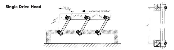
ROSTA oscillating mountings type AR in single rocker configuration: mounted on a round tube. It is best to adjust the desired center-distance between the axes on a surface plate and to subsequently tighten the clamp in order to frictionally connect the circular tube. The unit is fixed to the trough and the machine frame by means of frictional connection to the inner square section of the element by means of a bolt.
