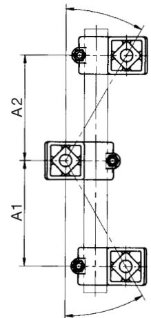
ROSTA oscillating mountings type AR in **boomerang configuration** for bidirectional conveying. The double rocker is mounted vertically, the middle element is rotated by 180°. The angles of the double rocker go in opposite direction, causing the material on the counterweight to move in opposite direction, too. The bidirectional conveying allows an easier processing of the bulk material, but still guarantees a perfect balancing of masses for high-speed oscillating conveyors.
