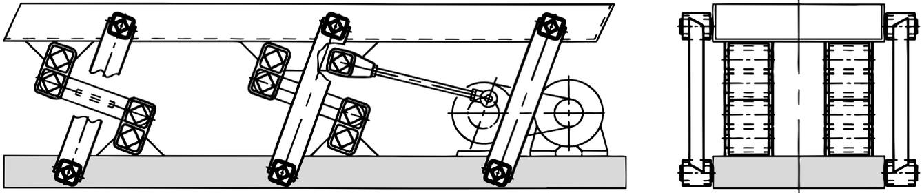
The oscillating conveyor systems are built such that they run very close to the resonance frequency in order to keep the energy consumption down and to improve the fatigue resistance of the structure (trough and frame). The total spring value  $c_1$  of the trough should be approximately equal to
