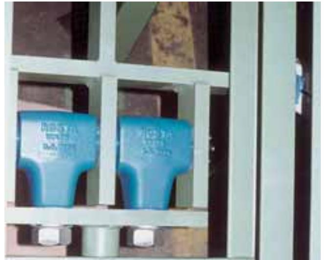
Drive head fixation on chip feeder
