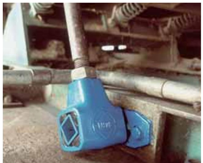
Rocker fixation on feeder frame
