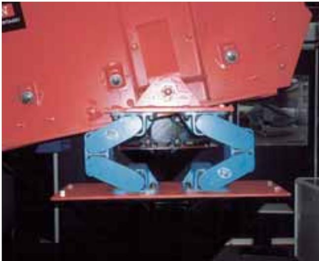
AB suspension of a circular gravel screen
