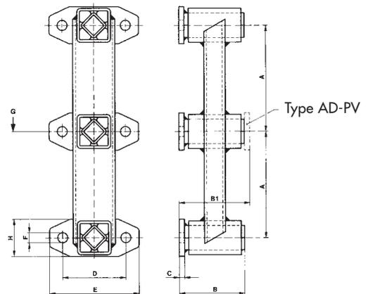
Type AD-PV with offset flanges
