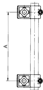
ROSTA oscillating mountings type AR in **single rocker configuration**: mounted on a round tube. It is best to adjust the desired center-distance between the axes on a surface plate and to subsequently tighten the clamp in order to frictionally connect the circular tube. The unit is fixed to the trough and the machine frame by means of frictional connection to the inner square section of the element by means of a bolt.
