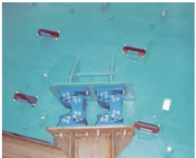
AB-D suspension of a dewatering screen
