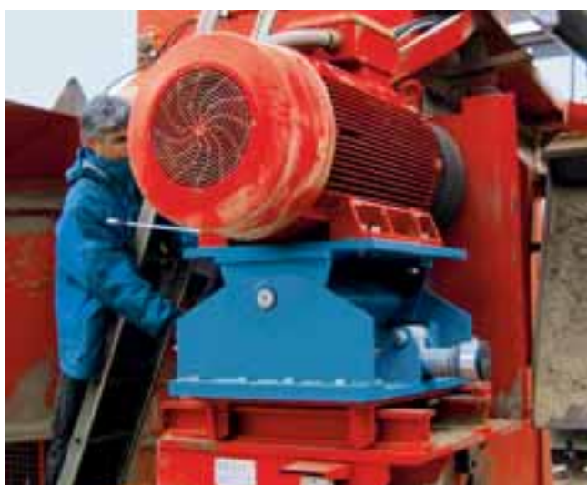
Elastic suspension of chipper-drive with MB 100
