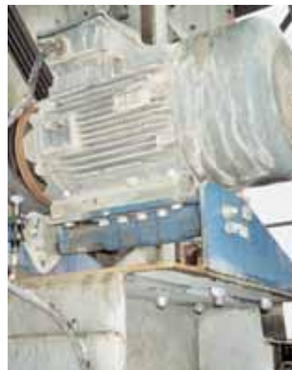
MB motor mount on dewatering screen
