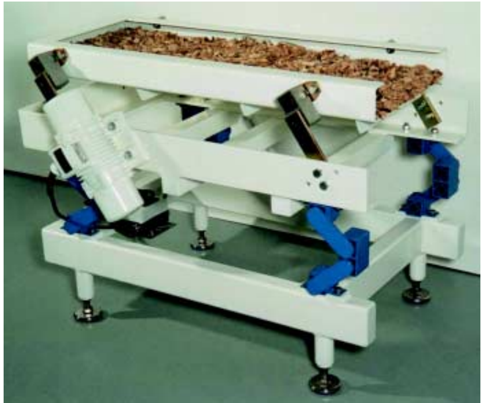
Demonstration conveyor trough for the ROSTA oscillating system „Silent Flow“ with chassis excitation (energetic amplification). Oscillating trough suspended on 4 AU-DO 27 rocker arms, chassis suspended on 4 AB 27; driven by 2 unbalanced motors. Machine frame is installed on 4 mounts NOX 70, M16.
