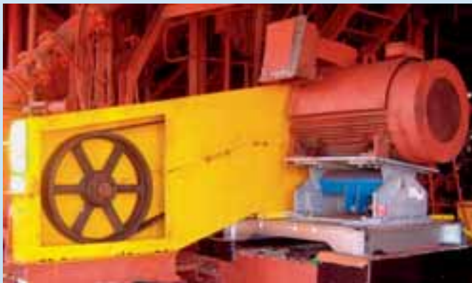
ROSTA motorbase type MB 100 with 220 kW drive motor for a Warman centrifugal pump.
