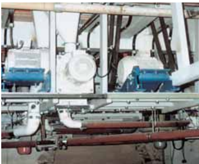
MB 50 with drives for roller mills
