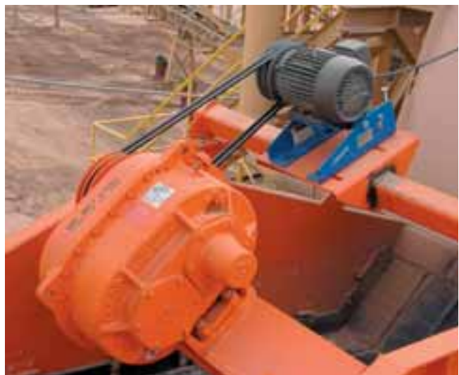
MB 50 with drive motor for exciter
