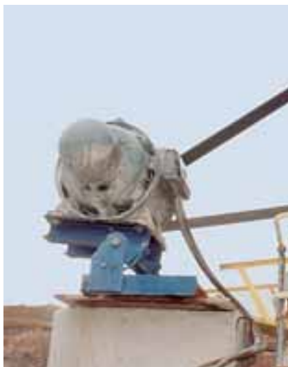
MB 70 motor mount in crusher
