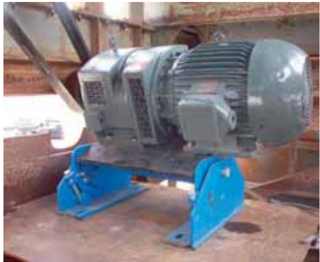
MB 70 with variable speed drive for crusher
