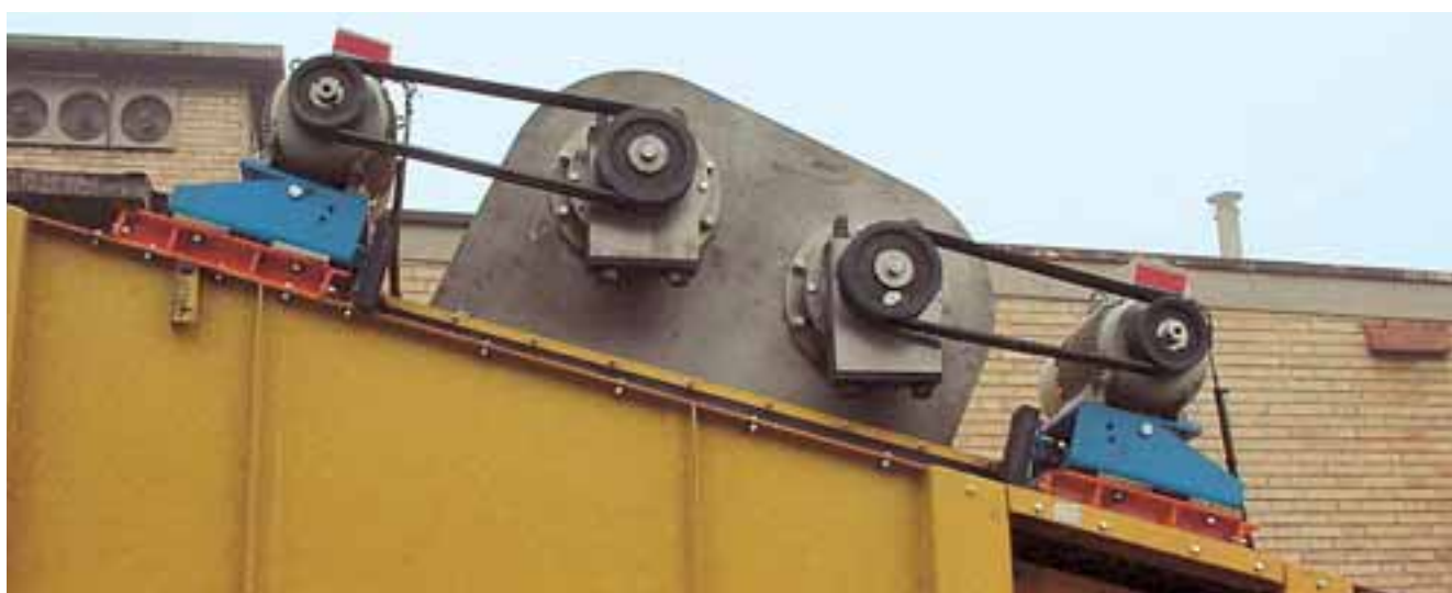
MB mounts of drives on asphalt screen
